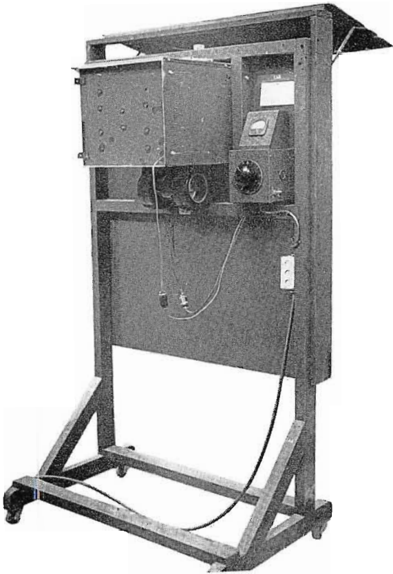
FIG. 6. Test chart transparency stand (rear view) shows lamp housing, auto-transformer and ammeter.
