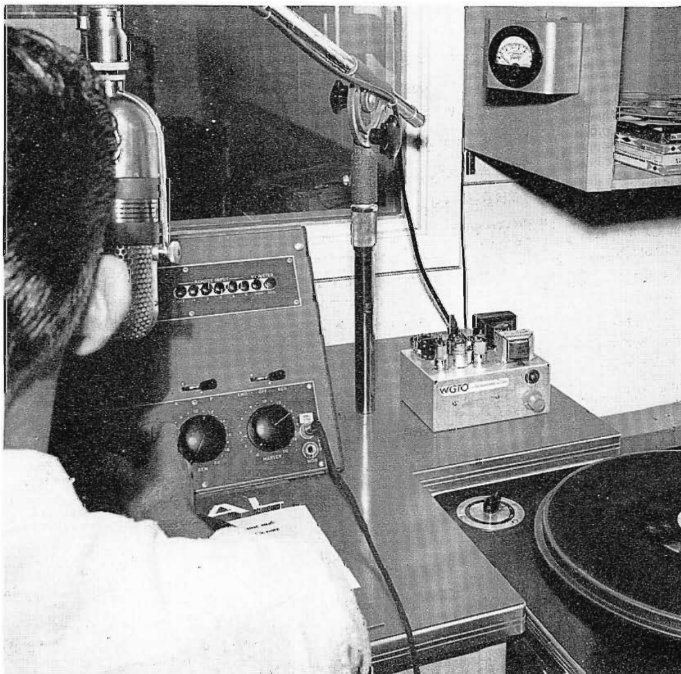
FIG. 4. Complete announcer timer is shown just to the right of the BC-2B Console. A brilliant light flashes, warning the announcer that his time is up.
